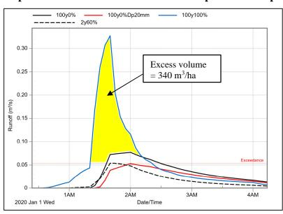
Graph 4: Unit Rate Peak Flows – Undeveloped vs Developed
