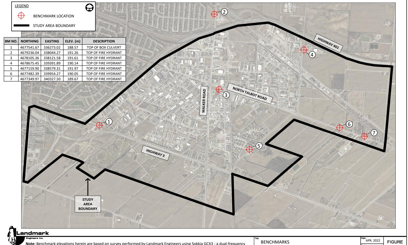
Note: Benchmark elevations herein are based on survey performed by Landmark Engineers using Sokkia GCX3 - a dual-frequency Global Navigation Satellite System (GNSS) receiver that provides Real-Time Kinematic (RTK) centimeter-level performance. These elevations are approximate, with a typical accuracy of +/- 5 cm.
