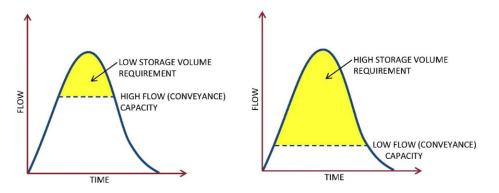
When considering issues of low conveyance capacity, the potential solution that typically first comes to mind is to increase this capacity with larger infrastructure. While this often can be a reasonable approach,
