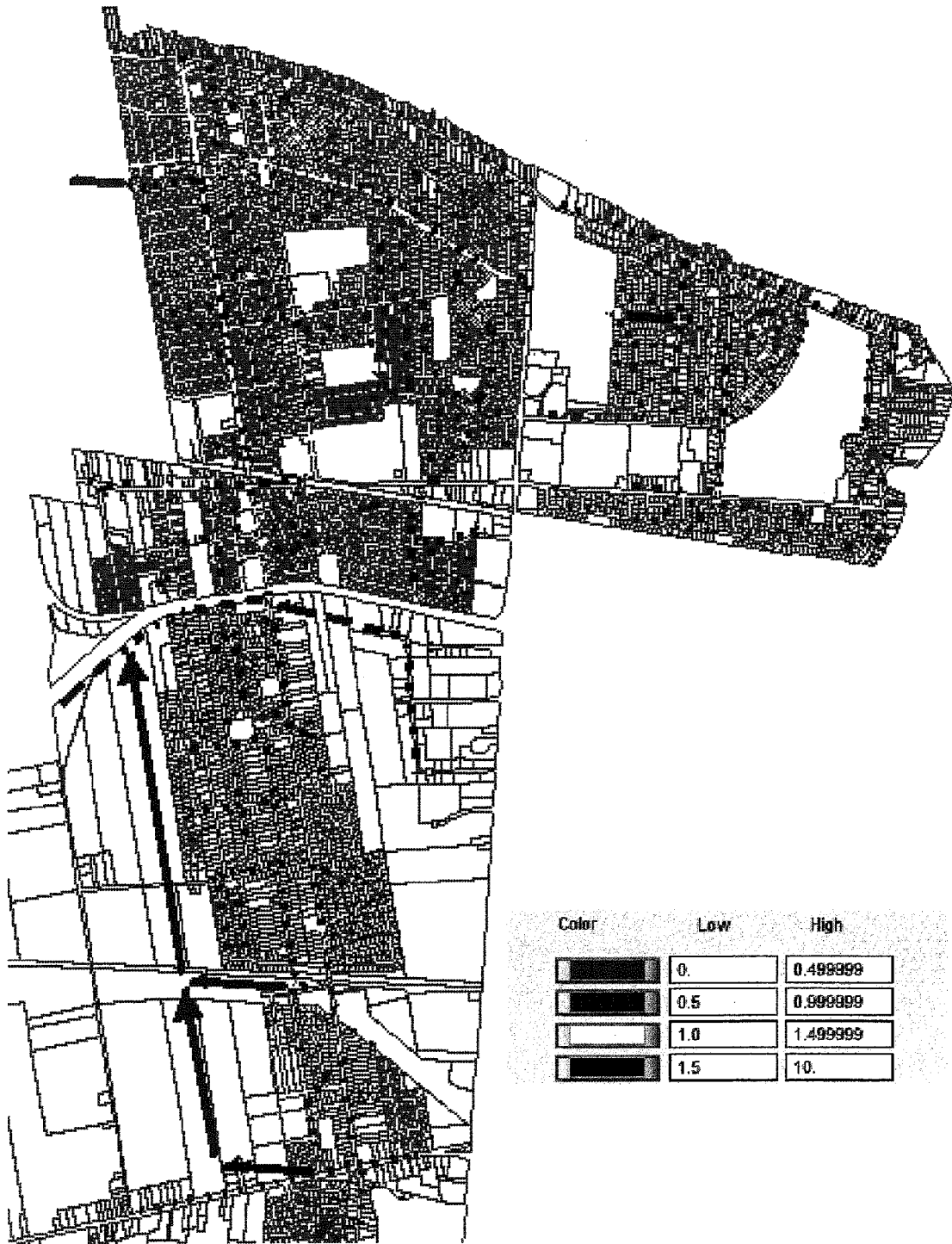
FIGURE 9: Scenario 2a – Graphical Encoding of the Ratio of Maximum Flow to Pipe Capacity
