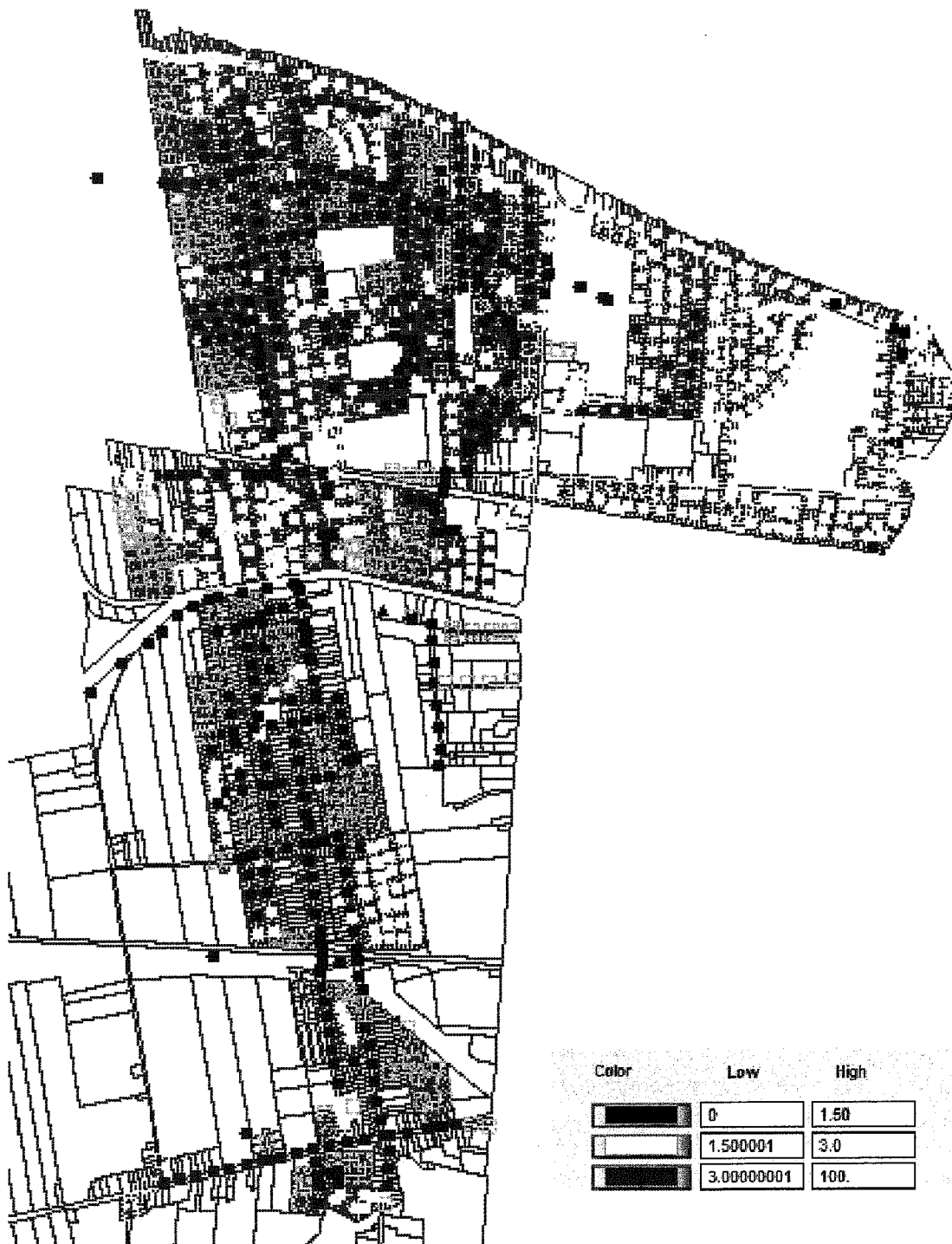
FIGURE 10: Scenario 2b – Graphical Encoding of the Depth of the Hydraulic Gradeline Below Ground
