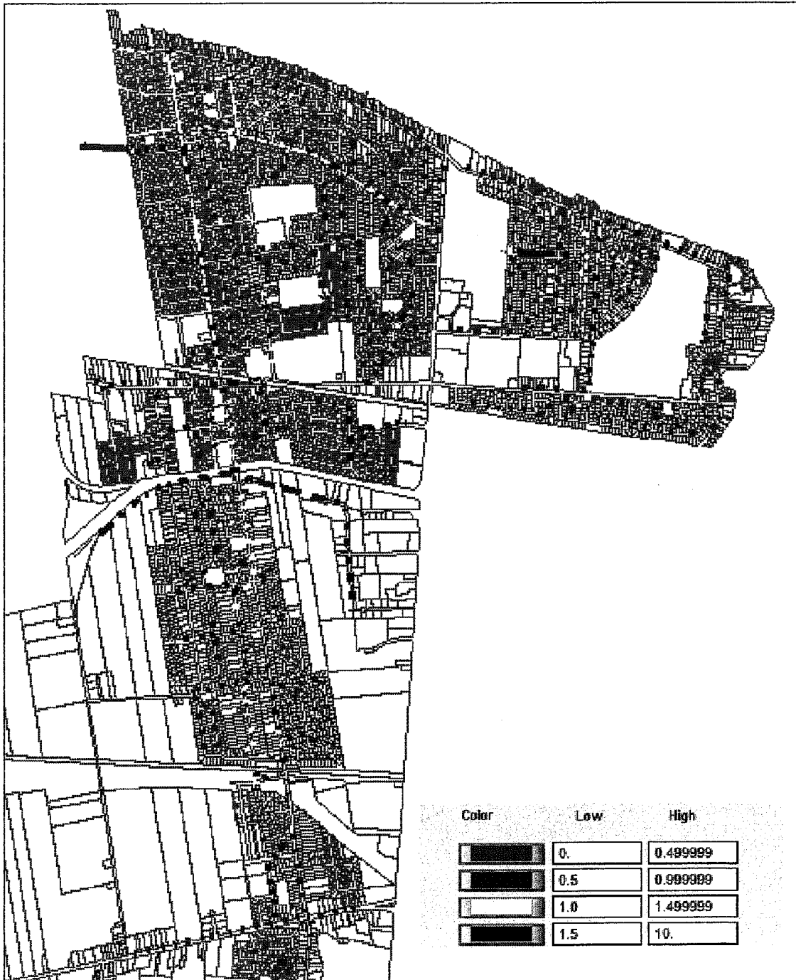
FIGURE 7: Scenario 1b – Graphical Encoding of the Ratio of Maximum Flow to Pipe Capacity
