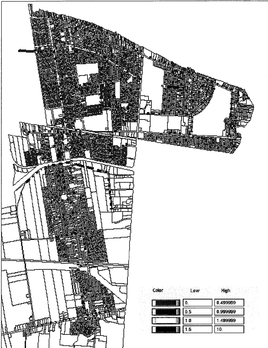
FIGURE 5: Scenario 1a – Graphical Encoding of the Ratio of Maximum Flow to Pipe Capacity
