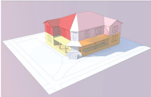
House converted to a fourplex, with parking spaces provided in the side / rear yard behind the house, and a common entrance
