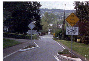
Mid-block narrowings Horizontal deflection; Curb extensions at mid-block locations
