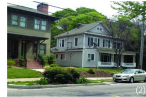
Curb extension Horizontal deflection; Extensions of the curbs into the travel lanes to narrow the street width
