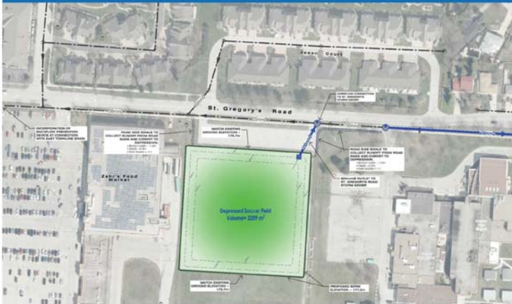
ALTERNATIVE 1 (aboveground storage outside of roadway)
