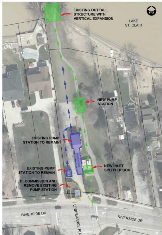
ALTERNATIVE 1 (Expansion of existing main pump station)
