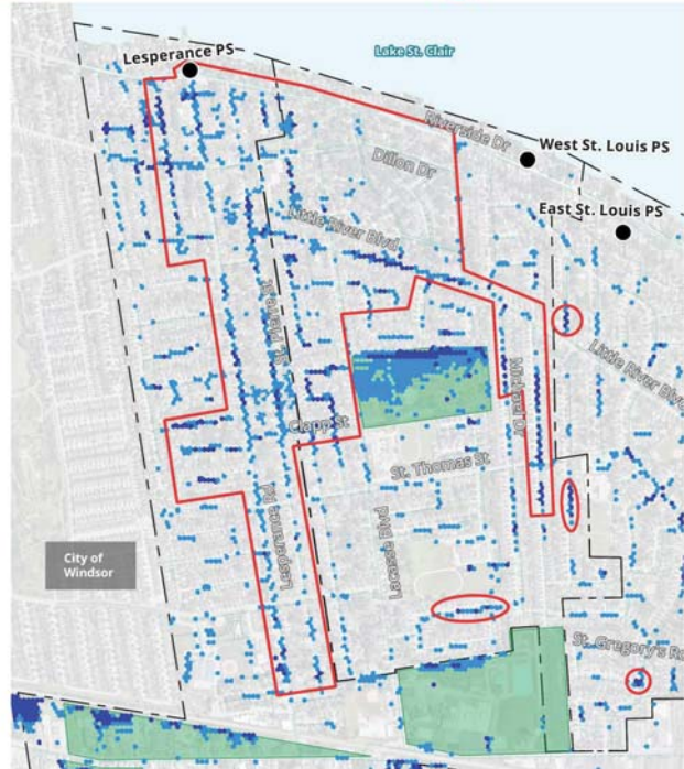
Existing Condition (1:100 Year Surface Ponding Simulation)
