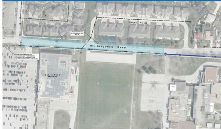
ALTERNATIVE 2 (underground storage within roadway)
