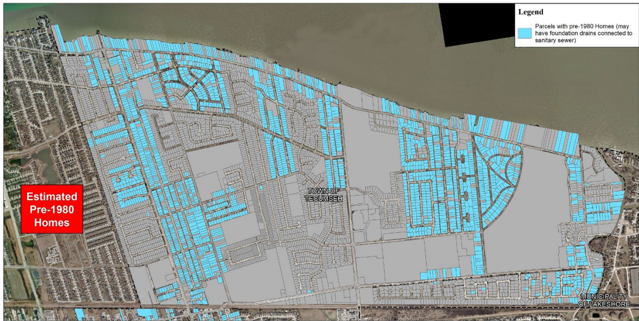
Figure 3.22 Estimate of Homes Constructed Prior to the 1980s with Potential Basement Drain Connection to the Sanitary Sewer
