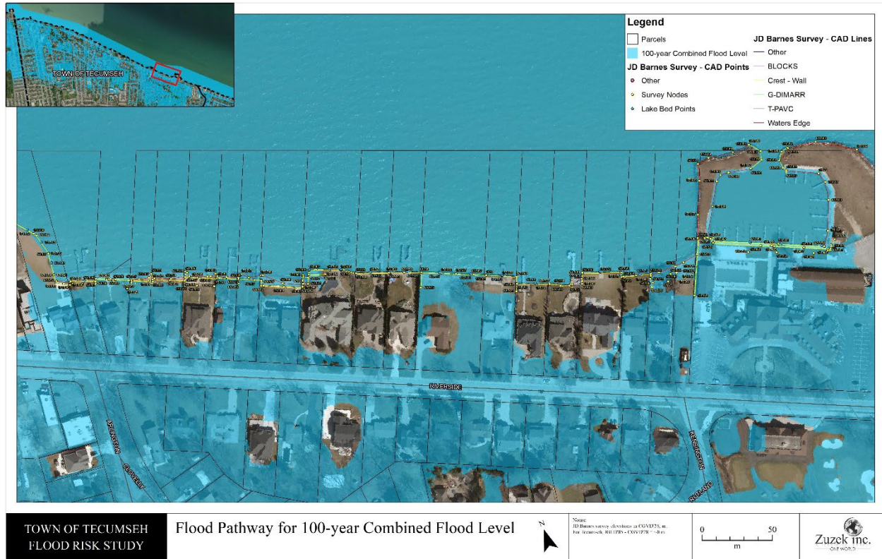
Figure 3.11 Flood Pathways for Wave Overtopping
