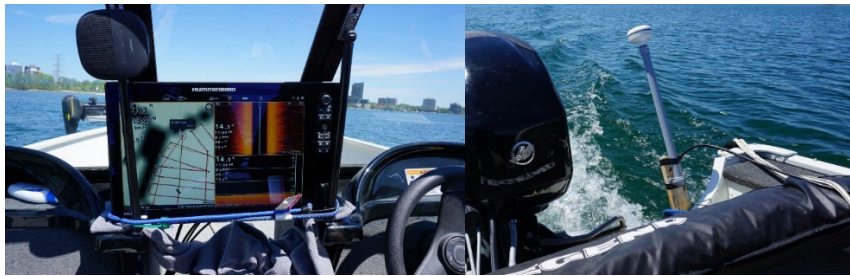
Figure 2.1 SOLIX Data Collection Unit and Transducer Mount
